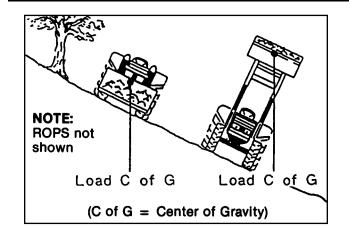
When working on side hills, **DO NOT RAISE LOADER TOO HIGH.** Keep an eye on terrain changes. Keep load low. Safety is a primary concern in the design and manufacture of our products. Unfortunately, our efforts to provide safe equipment can be wiped out by a single careless act of an operator.
