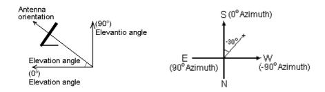
For example, in Shanghai, you can find out values of Elevation angle and Azimuth from Appendix F: Elevation angle=49 and Azimuth=-30. Then, put antenna face to up sky  $(49^{\circ})$  of southwest  $(-30^{\circ})$ .
