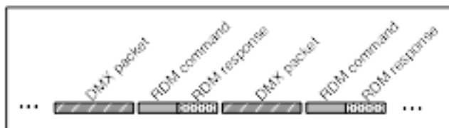
Figure 1 - DMX & RDM signal packet diagram
