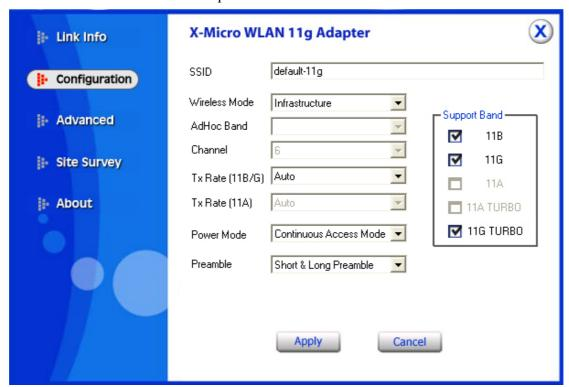
**SSID:** Service Set Identifier, which is a unique name shared among all clients and nodes in a wireless network. The SSID must be identical for each clients and nodes in the wireless network.
