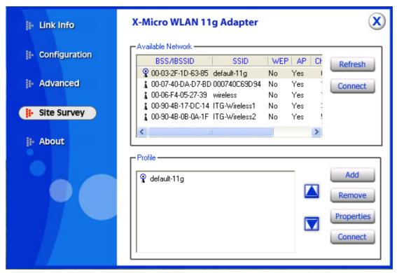
**Available Network** – displays the wireless networks (wireless clients and Access Points) that are in your signal range.
