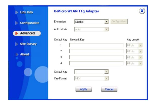
**Encryption:** 4 options are available: **Disable**, **Enable**, **WPA** and **WPA-PSK**. Select **Enable** or **Disable** for WEP data encryption feature. If one of the two options is selected, it is required to select the **Authentication mode** from the next dropping list. If **WPA** is selected, configuration is enabled. Please click the configuration. The below window is pop up. Then, please select the certificate that you like to use and enter the server name and login name
