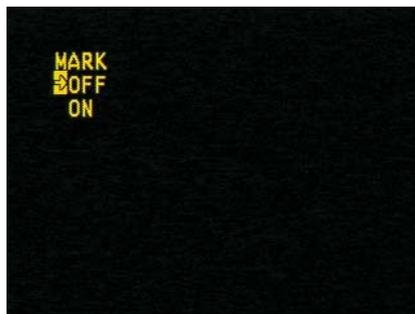
Select MARK with the Right Arrow. Then select OFF or ON with the Up and Down arrows. Select with the Right Arrow, and then back out to the main menu with successive presses of the Left arrow.
