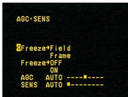
1. After following step A, B, and C on page 27 to bring up the main menu, use the down arrow to select AGC·SENS.
