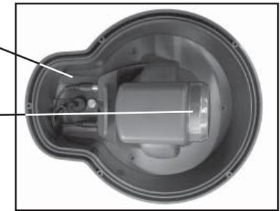
6. Remove the lens cap (Don't touch the lens).
