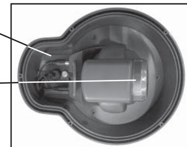
6. Remove the lens cap. (Don't touch the lens).
