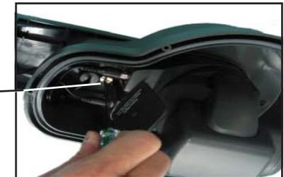
9. Point the pip on the camera's antenna in the direction of the TV that you connected the receiver to (if you're using the wireless feature).
