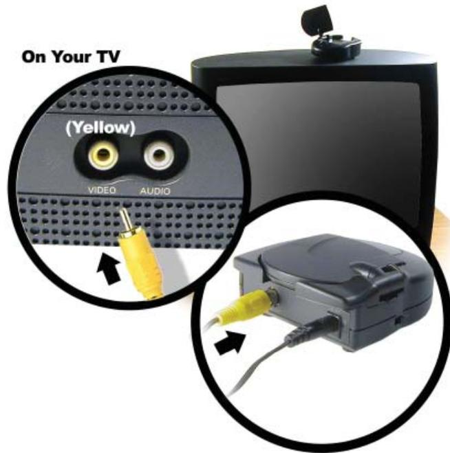
Connect the video cable into the video-out jack on the video receiver and into the video-in jack on your TV.
