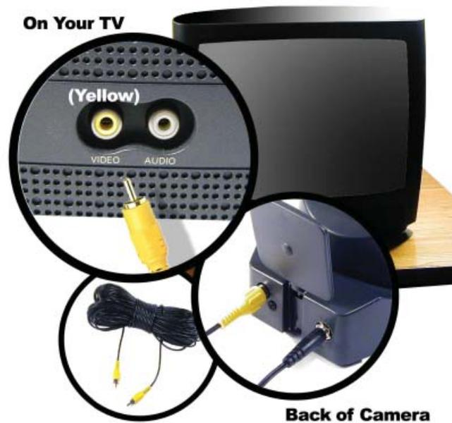
Turn on your TV and select its video input. Use the Video or Select buttons on your TV remote control, or try channel 0 and then Channel Down. The camera's picture should appear. Note, the picture will be upside down because the camera is intended to be mounted on a ceiling or overhang, after installing it into the dome. See page 22 if you want to flip the picture.
