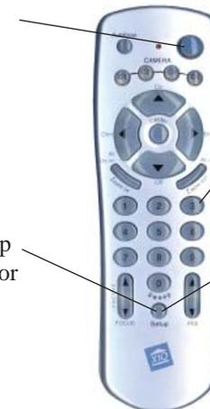
**Changing the camera's code:** Once you change the House Code on the remote control, you have to change the House Code on the SentinelPro Camera. Change the mode switch on the bottom of the camera to Program, then press the C1 button on the SentinelPro Remote Control. The camera is now set to the new house code. Put the mode switch back to Transmit Enable (or Transmit Disable if you are using the secure video connection).
