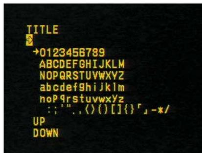
Use the Up and Down arrows to select the desired position on the screen (up/top or down/bottom). Then use the Up and Down arrows to select characters from the screen above, selecting each character with the Right Arrow. Then back out to the main menu with successive presses of the Left arrow.
