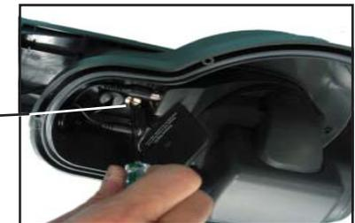
8. Attach the base of the dome to the mounting bracket. Then, tightly fasten the dome assembly to the bracket, by fixing the brass screw inside the dome.
