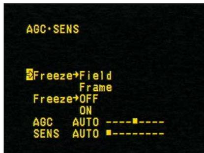
1. After following step A, B, and C on page 27 to bring up the main menu, use the down arrow to select AGC·SENS.
