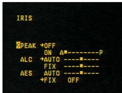
Use the up and Down arrows (On and Off) to select the desired menu item from the screen above right (Peak, ALC, AES). Then select the item with the Right Arrow. Adjust the item with the Up and Down arrows. Select with the Right Arrow, and then back out of the menu with successive presses of the Left arrow.
