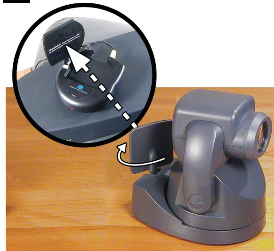
Once the camera and receiver are in place, adjust their antennas so that they face each other. The side of the camera's antenna with the dot on it should face the side of the receiver's antenna marked with four squares. Adjust the positions to improve the picture on your TV.
