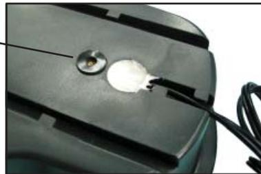
4. Attach the camera to the base of the dome using the brass screw on the outside of the dome's base.
