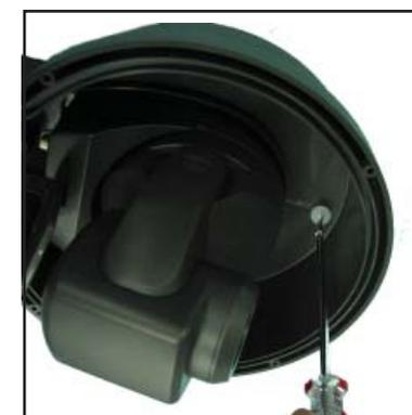
7. Attach the base of the dome to a ceiling by inserting three screws into the knockout holes on the inside of the base.
