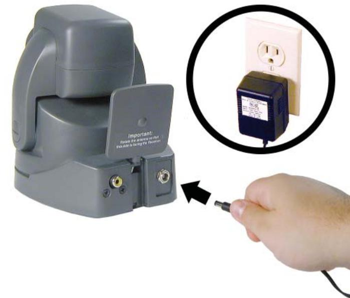
Plug the camera's power supply into a standard wall outlet. Plug the other end into the camera. Remove the protective cover from the camera's lens.
