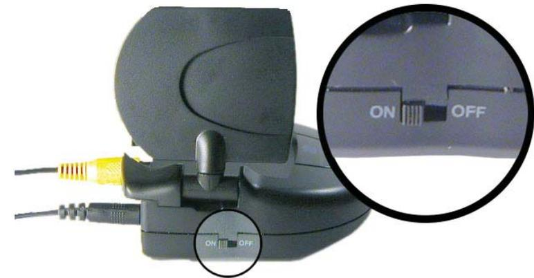
Make sure the power switch on the video receiver is set to "ON."
