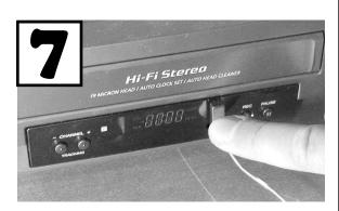
Press the emitter onto the VCR you are going to control, after removing the plastic from the adhesive backing.
