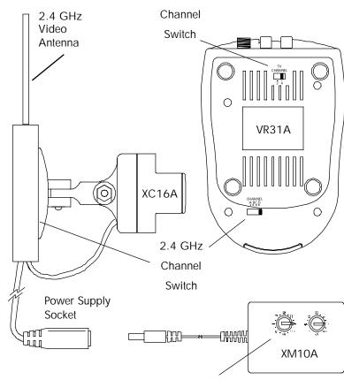
Used to set the code that the XM10A responds to, so you can turn the camera connected to it on and off by remote control (using X10 remote controls, sold separately).
