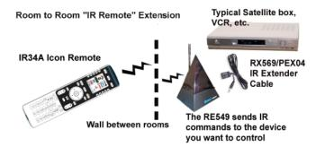
• Press any key on the remote. The RE549 receives the Radio Frequency (RF) signals and blasts the IR signals from its front face, or optionally through the RX569 emitter cable to control your IR compatible devices (TV, VCR, CD, etc.).
