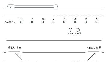
Connect to PC's serial port for computer control.
