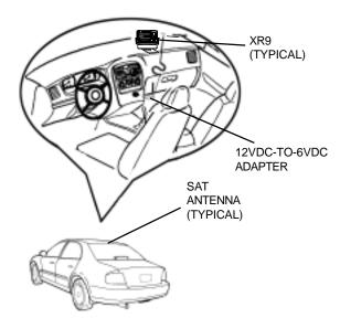
d. After determining the optimum position, turn off XR9 power, disconnect the power adapter from the vehicle cigarette lighter receptacle and disconnect the antenna cable.
