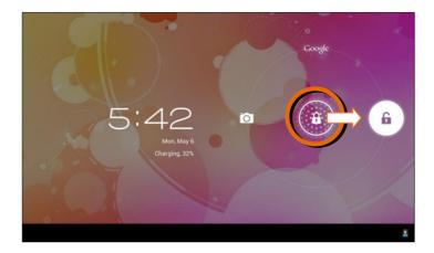
To unlock your XO Tablet in Android mode, touch and hold the **Lock** icon. When it turns into a circle drag it towards the right, to the **Unlock** icon.
