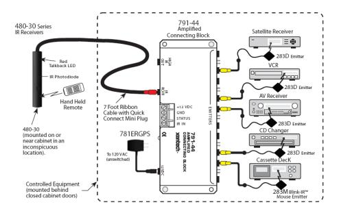
Since the IR receiver is in close proximity to the audio/video equipment, no wiring extension should be required so long as the connecting block is within reach of the 7-foot cable. The 3.5mm stereo type mini plug is connected to the "IR RCVR" jack on the Xantech Connecting Block.
