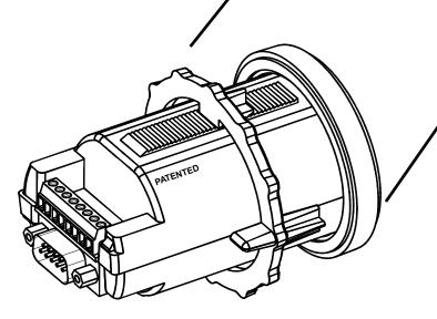
The gasket around the ring of the Link 10 should provide an adequate seal against moisture. If a sealant is used be sure it is **silicone** so that the Link 10 may be removed without damage.
