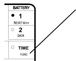
**FUNC:** The **FUNC** (Function) mode is used to set up special functions or features that are not commonly changed. They might be thought of as internal software switches that allow the selection of special functions, or values that, once set, are seldom changed.
