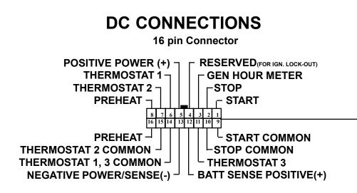
Connector view is looking into the AGS CONTROLLER. All wires should be #18 AWG MATING CONNECTORS: Xantrex P/N 76-0090-01 (mating connector and harness) is recommended for easy installation. Note: Connector below matches both AMP and MOLEX connectors, but pin numbers only match AMP connector. AMP: 770583-1, PINS 770988-1
