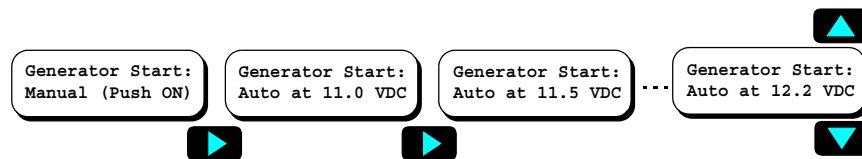
Figure 3-12 Generator Start menu items
