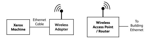
The Wireless Adapter (also known as an Ethernet-to-Wireless bridge) is a device that connects into the machine's Ethernet port using an Ethernet cable and acts as a wireless to wired Ethernet converter.
