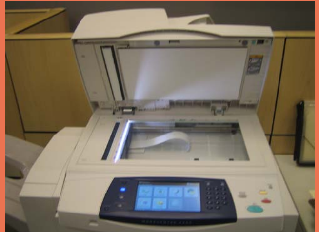
Above and below: The WorkCentre 4260's platen (above) and document feeder (below), with the document feeder's cover opened in order to expose the feeder's misfeed-access area.
