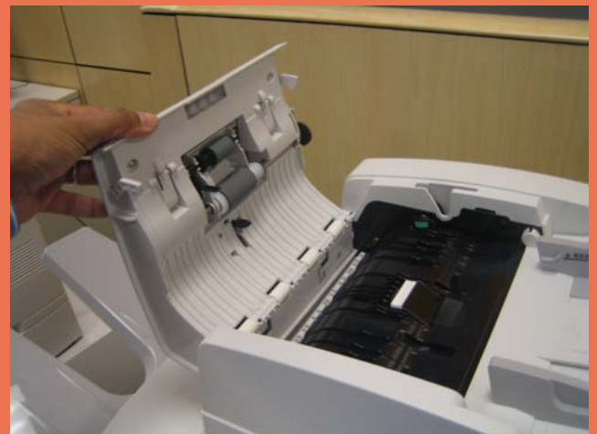
Above and below: The WorkCentre 4260's platen (above) and document feeder (below), with the document feeder's cover opened in order to expose the feeder's misfeed-access area.
