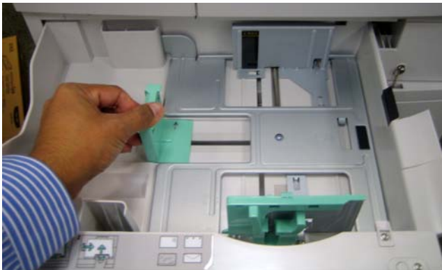
In order to adjust the paper drawers, the user must adjust the green rear guide by squeezing the lever and sliding it the guide into place to accommodate the desired paper size.
