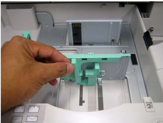
This paper tray is equipped with a side guide that the user must slide in order to adjust the desired paper width.
