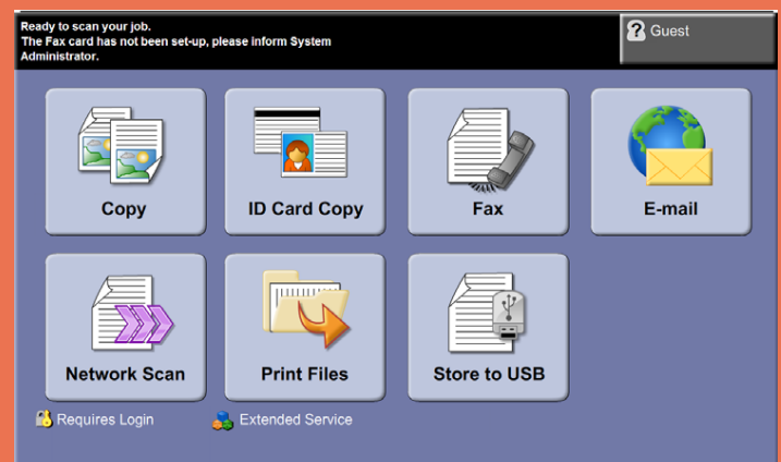
The "Services Home" button on the main control panel displays all of the device's available functions. Available options include Copy, ID Card Copy, Fax, E-mail, Network Scanning, Print Files, and Store to USB.
