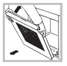
3. Grip the door on the two external sides and close it approximately half way. Pull the door towards you, lifting it out of its slot (*see diagram*).
