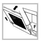
3. (With glass panel fitted to the inside of the door) Grip the door on the two external sides and close it approximately half way. Unlock the door by pressing on the clamps **F**, then pull the door towards you lifting it out of its seat (see diagram).
