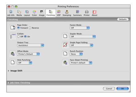
These print options are specific to the EX Print Server and the digital press. You must choose each Feature Set to see all the options. These options override settings in EX Print Server Printer Setup but can be changed from Command WorkStation.
