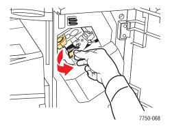
**3.** Remove the staple cartridge by lifting the gold handle.
