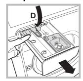
To pull out the dispenser drawer, open until the first stop point then press lever  $\bf A$  to open completely; finally, press one of the levers  $\bf D$  and pull the drawer outwards (see picture).
