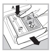
In order to fill the detergent and fabric softener tanks, the detergent dispenser drawer must be fully extracted: open the dispenser drawer up to the first stop point then press the lever (A) and open up to the second stop point, making sure that it is fully extracted. Avoid moving the dispenser
