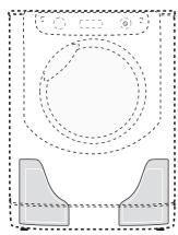
This washing machine is equipped with two tanks: one for liquid detergent (either concentrated or diluted) with a capacity of approx. 5.5 I and another for liquid fabric softener (either concentrated or diluted) with a capacity of approx. 3.5 I (see picture).
