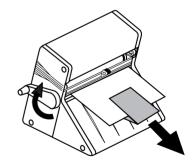
Install feed tray and trim off excess film using cut blade.
