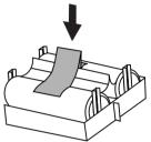
Insert partially used supply cartridge into dispenser. Note: tool should be positioned between rubber
