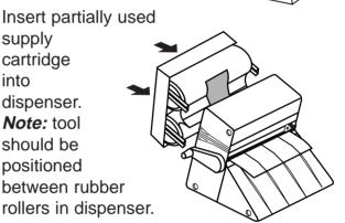
Turn handle clockwise until tool has exited dispenser and film is aligned and wrinkle-free.
