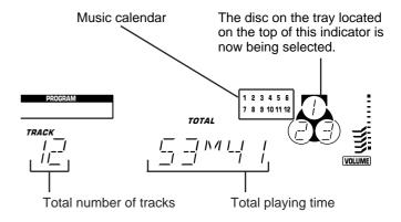
**5** If necessary, change the disc play mode by pressing the disc play MODE selector button on the remote control transmitter watching the display.
