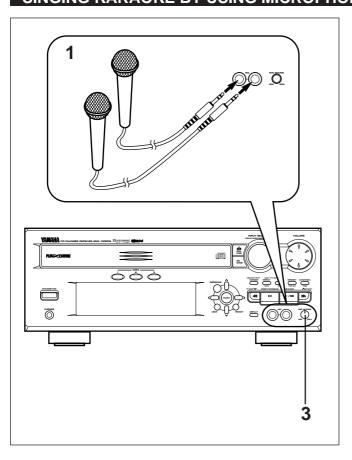
This unit is equipped with two MIC jacks and a MIC MIXING level control. These are available for singing karaoke or some other use.
