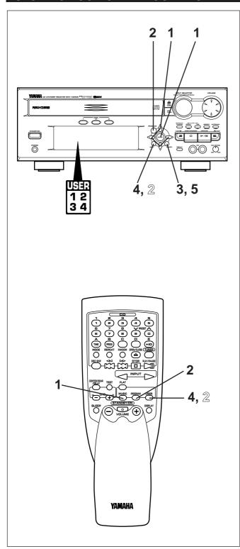
Your favorite pair of any equalizer mode (or an equalizer pattern of your own adjusting) and any sound field program can be stored as a user program. Up to 4 pairs can be stored as desired.
