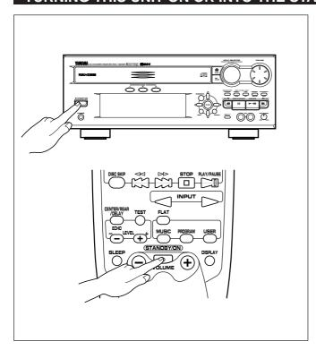
If the AC supply lead is connected to the AC outlet, this unit can be turned on and turned into the standby mode by pressing the STANDBY/ON switch on the front panel of this unit or the STANDBY/ON switch on the remote control transmitter.
