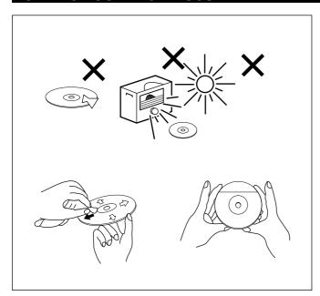
Compact discs are fairly resistant to damage, however mistracking can occur due to an accumulation of dirt on the disc surface.
