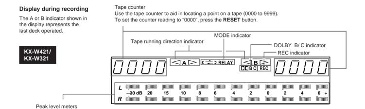
Indicate the peaks of the signal levels during recording and playback over a –30 dB to +6 dB range. There are separate meters for each left and right channel. These level meters have a peak hold function which holds the peak level for about 1.5 seconds.
