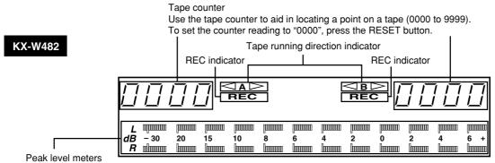
Indicate the peaks of the signal levels during recording and playback over a -30 dB to +6 dB range. There are separate meters for each left and right channel. These level meters have a peak hold function which holds the peak level for about 1.5 seconds.
