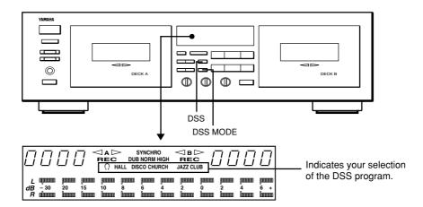
Pressing the DSS button turns on and off the DSS effect.
