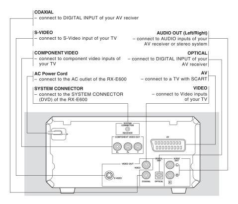
Caution: Do not touch the inner pins of the jacks on the rear panel. Electrostatic discharge may cause permanent damage to the unit.
