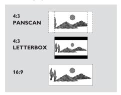
Select the aspect ratio of the TV to be connected. 4:3 PANSCAN → when you connect a normal TV to the DVD player. Displays the wide picture on the whole TV screen with a portion automatically cut off.
