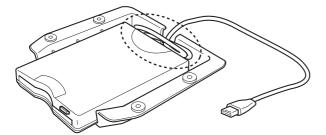
Attach the drive and case assembly to the left underside of the instrument, using the included four screws (4 mm x 10 mm).
