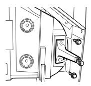
2 Attach and securely tighten the rear leg with the 92mm hexagon bolts.
