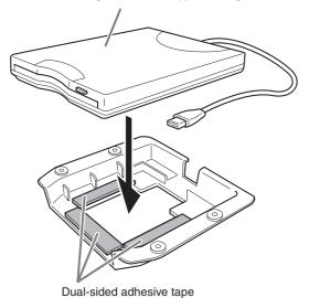
2 Fold the USB cable inside the case as shown.
