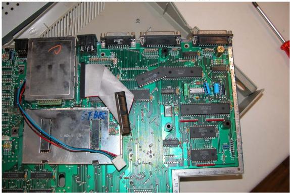
After soldering the dual in line FDD connector I've insert the plastic for the FDD Connector
