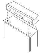
**3** Peel off the seal of the velcro strip with the smooth surface and apply to the positions determined in step 2.
