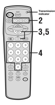
**3** Hold down SET and press  $\nabla$  until the transmission indicator lights.
