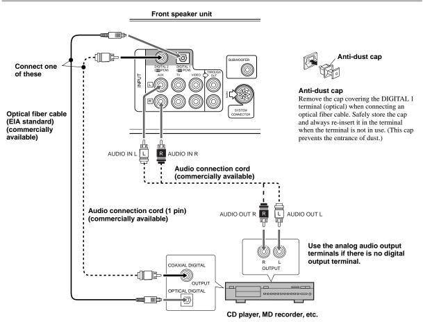
If the CD player or MD recorder has a digital output terminal, connect the optical or coaxial terminal on the CD player or MD recorder to the DIGITAL 1 (optical) terminal or DIGITAL 2 (coaxial) terminal on the front speaker unit using a commercially available optical fiber cable or audio connection cord (1 pin).
