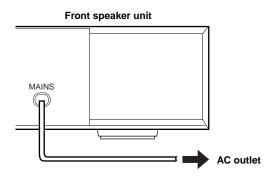
Once all connections have been made, check them one more time. Finally, insert the plug of the power supply cord for the front speaker unit into an AC outlet. Disconnect the power supply cord if you will not use the unit for an extended period.
