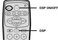
Press the DSP selector button (on the front speaker unit) or DSP (on the remote control).
