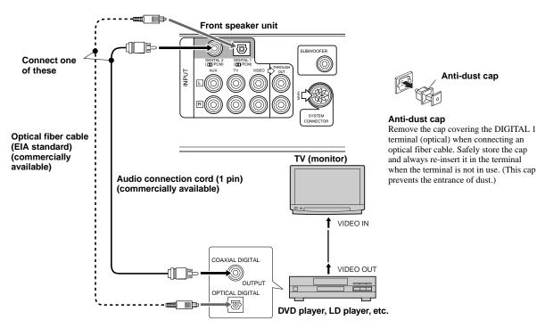
Connect the optical terminal or coaxial terminal of the LD or DVD player to the DIGITAL 1 (optical) terminal or DIGITAL 2 (coaxial) terminal of the front speaker unit using a commercially available optical fiber cable or audio connection cord (1 pin).
