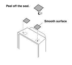
4 Align both the velcro strip on both sides and firmly press downward on the top of the front speaker unit.
