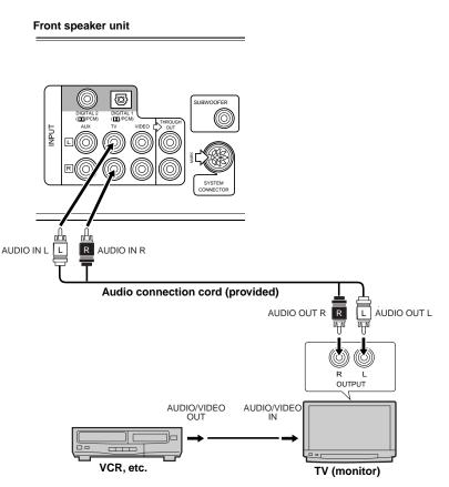
Connect the audio output terminal on the TV (monitor) to the TV terminal on the front speaker unit using the provided audio connection cord.
