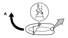
B. Less throttle produces lower thrust, so the watercraft will turn more gradually.
