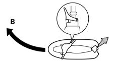
C. Releasing the throttle lever completely produces only minimum thrust. If you are traveling at speeds above trolling, you will have rapidly decreasing ability to steer without throttle. You may still have some turning ability immediately after releasing the throttle lever, but once the engine slows down, the watercraft will no longer respond to handlebar input until you apply throttle again or you reach trolling speed.
