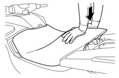
(2) Install the rear seat. Make sure that the seats are securely installed before operating the watercraft.
