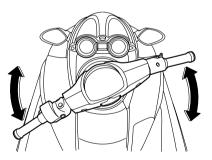
Pull the handlebars up and down to check that the lock lever and handlebars are locked in place. (See "Telescopic steering system" on page 33 for more information.)
