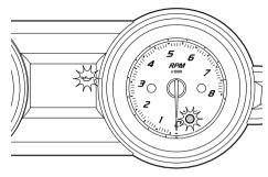
If this occurs, immediately reduce the engine speed, return to shore, and then check the engine oil level. (See page 50 for engine oil level checking procedures.) If the oil level is sufficient, have a Yamaha dealer check the watercraft.
