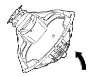
(2) Remove any weeds or debris from around the jet intake, drive shaft, impeller, jet pump housing, and jet thrust nozzle.
