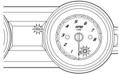
If this occurs, immediately reduce the engine speed, return to shore, and have a Yamaha dealer check the engine.
