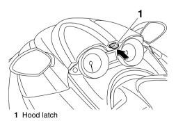
To close the hood, push down on the rear of the hood until it latches securely. Make sure that the hood is securely closed before operating the watercraft.
