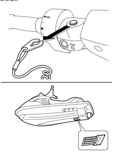
(1) Place a suitable clean cloth or carpeting underneath the watercraft to protect it from abrasions and scratches. Turn the watercraft on its side as shown. NOTICE: Always turn the watercraft over onto its port (left) side. When turning the watercraft on its side, support the bow so that the handlebars are not bent or damaged. [ECJ00061]
