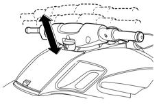
(2) Check that the lock lever returns to its original position and that the handlebars are locked in place.
