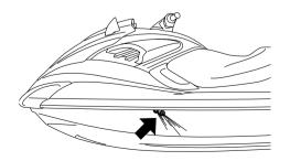
To check for proper operation of the cooling system, check that water is being discharged from the port (left) pilot outlets. If water is not being discharged from these outlets, cooling water may not be circulating in the engine. When this occurs, stop the engine and check for the cause. (See pages 41 and 88 for more information.)
