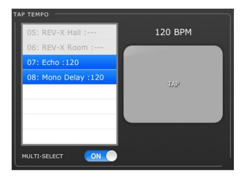
Select the relevant effect from the list of 4 effects in the left side of this section. Effects which do not have a BPM parameter will be greyed out and cannot be selected.
