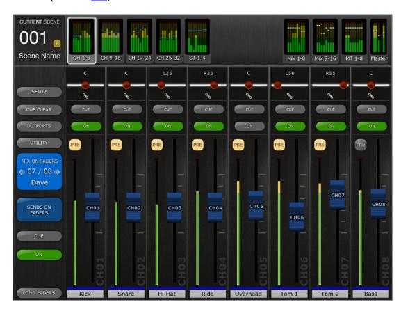
The large [MIX ON FADERS] button displays the currently selected Mix Bus number and its name. The color of this button matches those used in the M7CL console.
