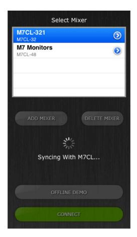
The message "Syncing With M7CL..." will appear while StageMix is obtaining parameters from the console. After this process is complete, the Mixer window will appear and StageMix is ready to be used.
