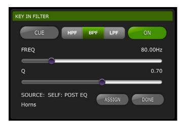
[CUE]: Tap this button to Cue the Key In signal [HPF]/[BPF]/[LPF]: Select the Key In Filter type among these choices. [ON]: This button is used to activate the Key In Filter.
