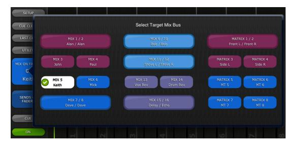
Choose the "Target Mix Bus" from Mix 1-16 and Matrix 1-8. The currently selected Mix will appear as a white button with a check mark. Stereo pairs appear as single large buttons.
