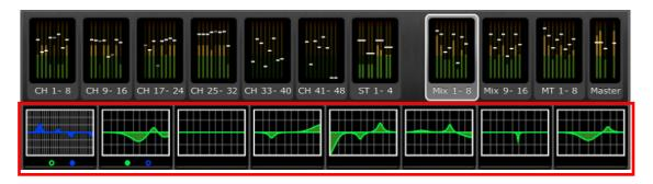
Green and blue dots below each EQ curve indicate the types of EQ available on that channel, and the type of EQ (PEQ or GEQ) that is currently displayed for that channel. A green dot indicates PEQ and a blue dot indicates GEQ. When only PEQ is currently available on a channel, no dots will appear below the curve. (In Demo mode, GEQs appear on Mix busses1, 7 and 8).
