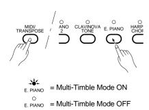
The Multi-Timbre mode is a special mode in which the Clavinova voices can be independently controlled on different MIDI channel numbers (1 through 10) by an external MIDI device such as the Yamaha DRC-20 Disk Recorder. The Multi-Timbre mode can be activated as follows:
