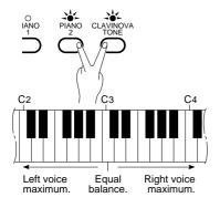
The volume levels of the two voices combined in the DUAL mode are normally set automatically to produce a pleasing balance (see "Default Settings" below). The balance can be adjusted manually by using the C2 through C4 keys on the keyboard while pressing the two voice selectors corresponding to the voices to be combined in the DUAL mode.
