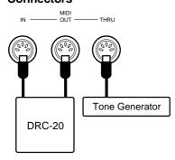
The MIDI IN connector receives MIDI data from an external MIDI device (such as the DRC-20 Disk Recorder, or DOM-30 Disk Orchestra Module) which can be used to control the Clavinova. The MIDI THRU connector re-transmits any data received at the MIDI IN connector, allowing "chaining" of several MIDI instruments or other devices. The MIDI OUT connector transmits MIDI data generated by the Clavinova (e.g. note and velocity data produced by playing the Clavinova keyboard).
