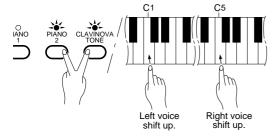
Depending on which voices you combine using the DUAL mode, the combination may sound better if one of the voices is shifted up an octave. To shift the right voice, press the C5 key while pressing the two voice selectors corresponding to the voices to be combined in the DUAL mode. Press C5 again to shift the voice back to its normal range. Use the C1 key in the same way to shift the left voice.
