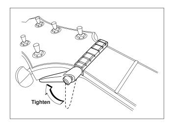
7 This completes locking block replacement. Install the new strings and tune the guitar. (Refer to the "Installing the new strings" section in the FC Tremolo System Manual.) Free Manuals Download Website
