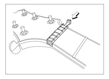
6 Re-attach the locking lever and tighten lightly.
