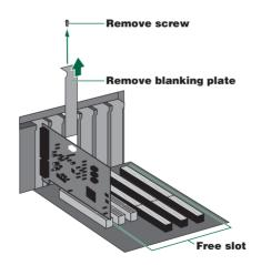
**5** Insert your SCSI adapter card into the slot using both hands. Make sure it is seated firmly in the slot. Then secure the card by replacing the screw used for the blanking plate.
