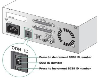
The SCSI ID number for each device on the chain must be unique. Make sure the CRW6416SX drive's SCSI ID number is not the same as that of any other device on the chain. By factory default, the CRW6416SX is assigned ID number "1" but this can be changed.
