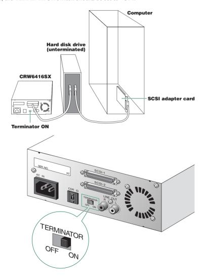
**ENOTE** By factory default, the Terminator switch is set to "ON."
