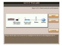
7 Press the [G](NEXT) button to search for wireless network near the instrument.
