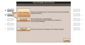
**5** Press the [B] button to select "LAN cable," then press the [G] button to proceed to "NEXT."
