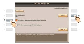
Make sure that the devices are connected as shown in the illustration of the display, then press the [G] button to proceed to "NEXT."
