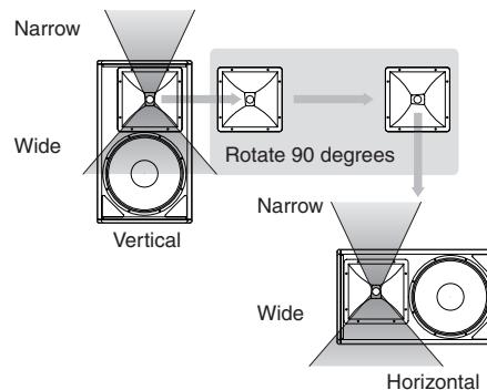
**NOTE** If you use the speaker as a floor monitor, change the horn dispersion so that the upward spread is wide and the downward spread is narrow, as shown in the diagram.
