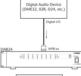
In this example, the DA824 sources the wordclock signal automatically from the WORD CLOCK IN connector.
