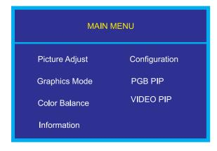
These submenus can be accessed using the Up and Down buttons on the display panel. See sections below for specifics regarding the submenus.
