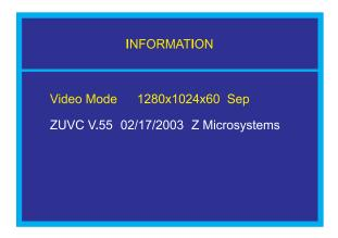
Within this submenu, view the video mode resolution, the refresh rate, and the sync mode. Press "Exit" to return to the Main Menu. The Firmware Version and Build Date are also available on this screen.
