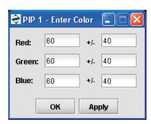
Any combination of values for the three base colors can be entered in the fields to the left. Each color value can be set between 0 and 255 on the RGB color range. For example, if all three colors are set to "0" the result will be black. This value acts as a center point to the values entered in the offset field. The offset value to the right is the amount the software will offset the centerpoint color values from one another to create color differentiation.
