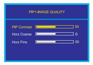
Within this submenu, highlight the item to adjust, and use the Left and Right buttons to alter the PIP Contrast, the Horz Coarse and the Horz Fine characteristics. Press "Exit" to return to the RGB PIP submenu. The new adjustments will be applied automatically.
