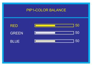
Within this submenu, highlight the color to adjust, and use the Left and Right buttons to alter the Red, Green and Blue color characteristics.
