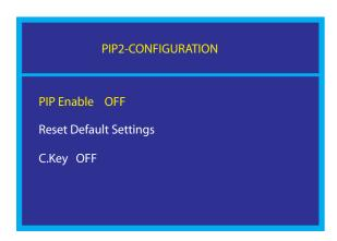
Highlight the "PIP Enable" option and press the Left or Right buttons to choose the "ON" option. The PIP screen will appear. Exit the "PIP Configuration" submenu by pressing the "Exit" button.
