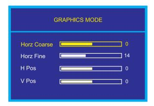
"Graphics Mode" is used to adjust the positioning of the image. Use the Up and Down Keys to highlight the desired option. Use the Left and Right buttons to adjust the following modes: Horz Coarse, Horz Fine, H Pos, and V Pos.
