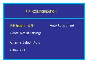
Highlight the "PIP Enable" option and press the Left or Right buttons to choose the "ON" option. The PIP screen will appear. Exit the "PIP Configuration" submenu by pressing the "Exit" button.
