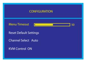
The StarGate has two channel options. Highlight "Channel Select" and use the Left and Right keys to change channels. If both channels have been configured for use, the following options are relevant:
