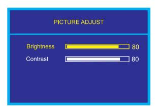
Use the Up and Down Keys to highlight the desired option. Use the Left and Right buttons to increase and decrease the Brightness and Contrast characteristics of the screen. Press "Exit" to return to the Main Menu. The new adjustments will be applied automatically.
