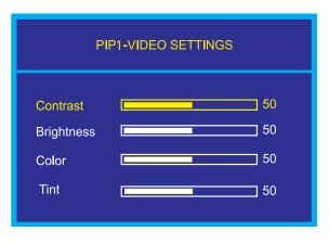
Within this submenu, highlight the item to alter, and use the Left and Right buttons to adjust the Contrast, Brightness, Color and Tint characteristics.
