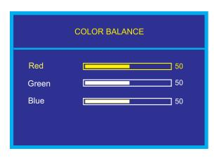
Use the Up and Down Keys to highlight the desired option. Use the Left and Right buttons to adjust the colors of the screen image.
