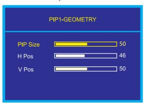
Within this submenu, highlight the item to alter, and use the Left and Right buttons to adjust the PIP size, the Horizontal Positioning and the Vertical Positioning. Press "Exit" to return to the RGB PIP submenu. The new adjustments will be applied automatically.
