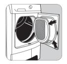
Clean periodically the interior part of the door to remove any fluff from the seals around the filter. Accurate cleaning ensures correct drying.
