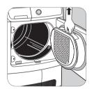
The filter in the inner door must be removed for cleaning. Do not be alarmed by the amount of fluff. It is not due to excessive wear caused by the dryer. All fabric loses fluff when drying but it goes un-noticed in the air. In a tumble dryer it simply collects in the filter. After a while, a whitish patina due to detergent residue on laundry forms on the fil-
