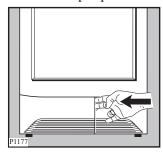
To pull out the condenser, first turn the two red stops inwards as shown and then remove the condenser unit holding it at the handle.
