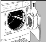
The filter in the inner door must be removed for cleaning.
