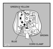
The wire coloured green and yellow must be connected to the terminal marked with the letter «E» or by the earth symbol  $\frac{1}{2}$  or coloured green and vellow.
