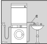
If the appliance is stacked on the washing machine, the condensed water can be discharged through the hose as shown in figure, but take into account that the hose must be pointed downwards.
