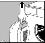
You should not be alarmed by the amount of fluff which collects on the filter; this is due to normal wearing of the fabrics dried and not to incorrect operation of your machine. Rubbing of the fibres during normal wear and washing forms fluff. If laundry is dried on a line, this fluff simply flies away, whereas inside the tumble dryer it collects together and swells considerably as a result of the drying action.
