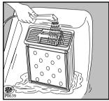
Also clean the outside, removing all fluff. Clean the rubber seal round the porthole door and the seal of the condenser in the inner door with a damp cloth.
