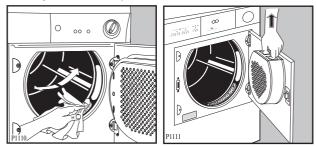
The filter in the inner door must be removed for cleaning.
