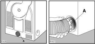
Advice: If the hose is long and the room temperature low, the moisture might condense to water inside the hose. This is an unavoidable natural phenomenon. To prevent this water from lying in the hose or flowing back into the tumble dryer, it is advisable to drill a small hole (dia. 3 mm) in the lowest point of the hose and to place a small container below it.(See picture, point B).
